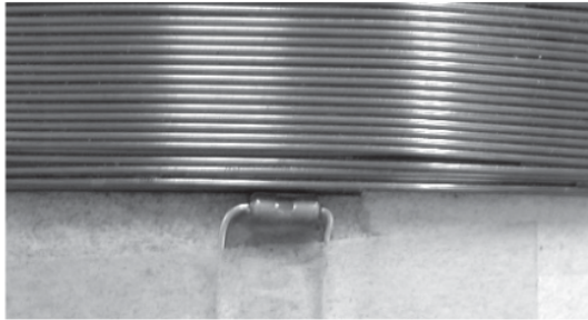
Heat sensor on voice coil
